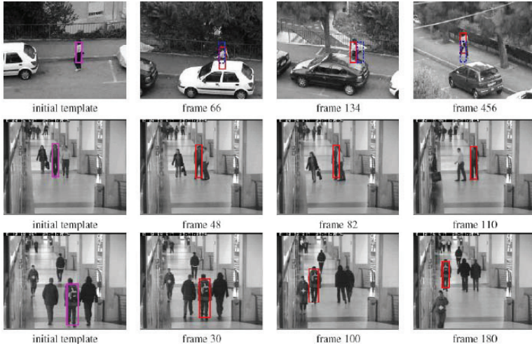
Fig. 9. Results from Tracker-3 (courtesy from (Adam et al.,06)): results from Tracker-3 (Red); manually selected target (Pink). Top to bottom: frames from the videos "walking lady", "OneShopOneWait2Cor" and "ThreePastShop2Cor".
