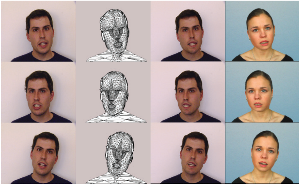
Fig. 11. 3D facial expression analysis. The left column shows example frames of the original sequence. Facial expression parameters of a deformable face model are estimated. The second column shows the animated mesh, while the third column depicts the textured model. The rightmost column refers to expression cloning where the deformation parameters are mapped onto a different person's model.
