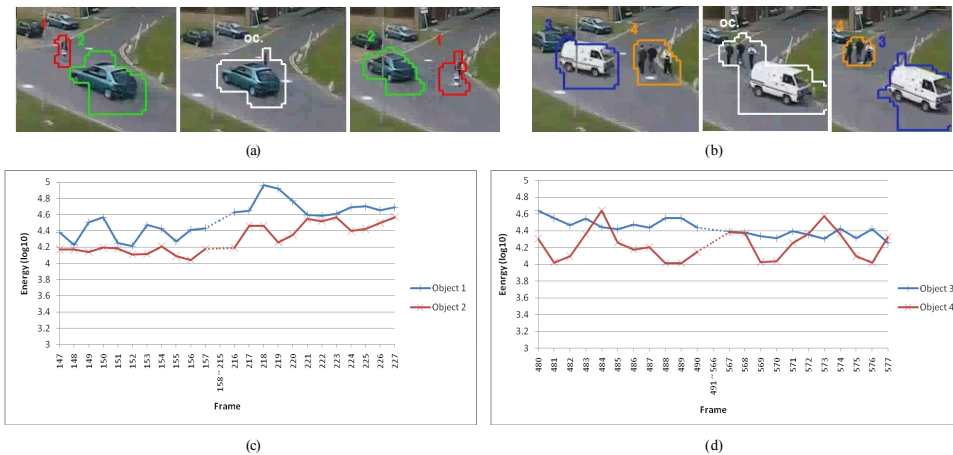
Fig. 2. Computing energy similarity of two occluded objects in PETS2001 sequence (a) between object 1 and object 2, (b) between object 3 and object 4. Graphs show the value of energy of (c) objects 1 and 2, (d) object 3 and 4. Dashed lines in the graphs imply the occlusion.
