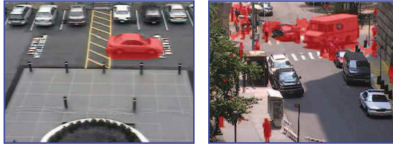
Fig. 2. Keyframes of example videos. (a) Sparse traffic scene; (b) Crowded activity scene. Red overlaid regions in the image represent the areas occupied by foreground moving objects.
