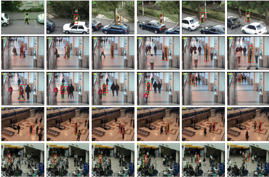
Fig. 11. Comparing tracking results from 2 trackers: the hybrid tracker (red solid line box) and the JMSPF tracker with online learning (green dash line box). From rows 1-5: result frames (key frames) from videos "walking lady", "OneShopOneWait2Cor", "ThreePastShop2Cor", "Pets2006_S5_C4" and "Pets2007_DS5_C1".
